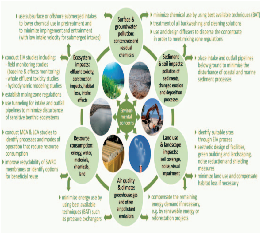
Figure 2.26 Key environmental concerns of seawater desalination projects and measures for impact mitigation.
